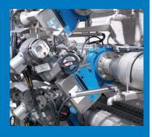
and improve inlet flow paths for accurate flow measurements. Egger will supply the ABB Sensy-Master thermal mass flow meter hard mounted one (1) diameter upstream to ensure compact design with industry leading 1-2% accuracy, repeatability, and 0.5 second response time.
