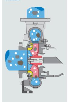
solids. The blade leading edge and the opposing wear plate have special designs that make it possible to transport even long-fibre components, such as occur in wastewater.
