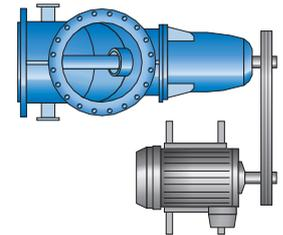
Motor to one side on a tensioning bar
