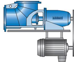
Universal joint drive with spur gear
