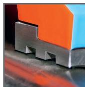
by means of a narrow gap. This is a cost-effective seal version for pumped media containing solids when a flushing liquid can be used.
