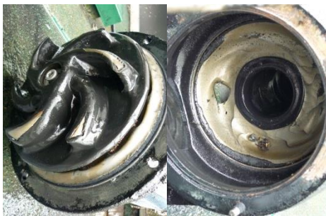
Impeller and casing of pump with rubber lining casting
