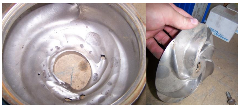
Figure 1 Hard chrome (1.4313 / <320HB = 34HRC) is not hard enough
