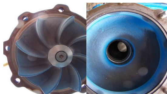
Pump made of chrome molybdenum chilled casting Figure 3 Start of test 06/2007
