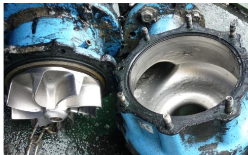
Pump made of chrome molybdenum chilled casting
