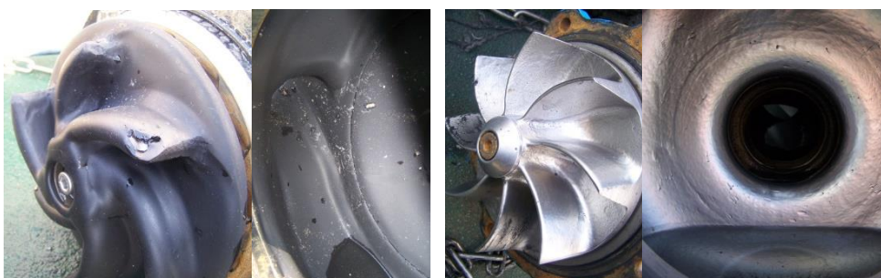
Impeller and casing of pump with rubber-lining casting
